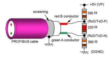
Figure 3: Internal Termination Resistors
