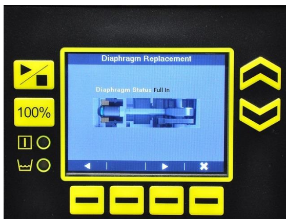
Figure 31: Diaphragm Replacement (Full In)
