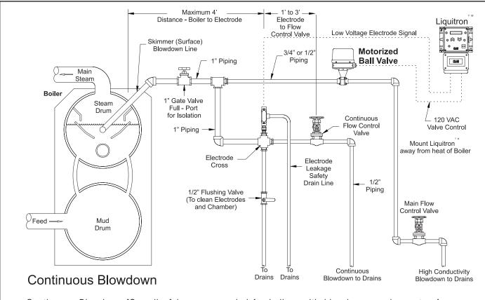
Continuous Blowdown [Sampling] is recommended for boilers with blowdown requirements of over 5,000 lbs/hr. This system allows for continuous monitoring and control of boiler water conductivity.
