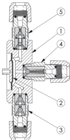
The AUTOPRIME™ liquid end consists of 5 functional elements. They are the Head (1), Diaphragm (2), Suction Check Valve (3), Discharge Check Valve (4) and Autoprime Valve (5).
