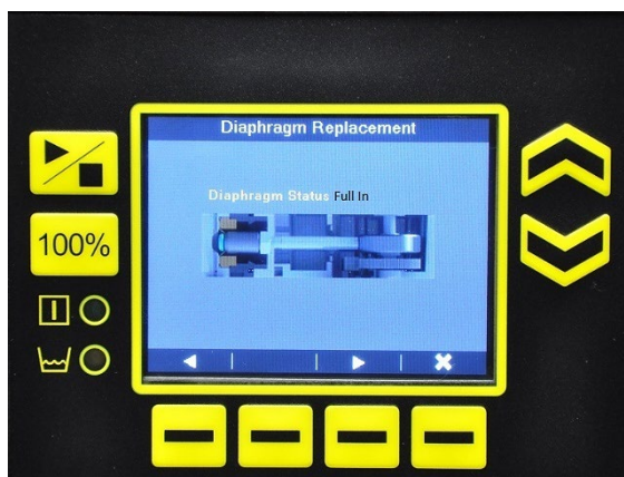
Figure 33: Diaphragm Replacement (Full In)
