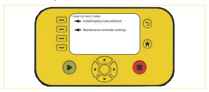
Press the soft button for Install new tube element to enter maintenance mode.
