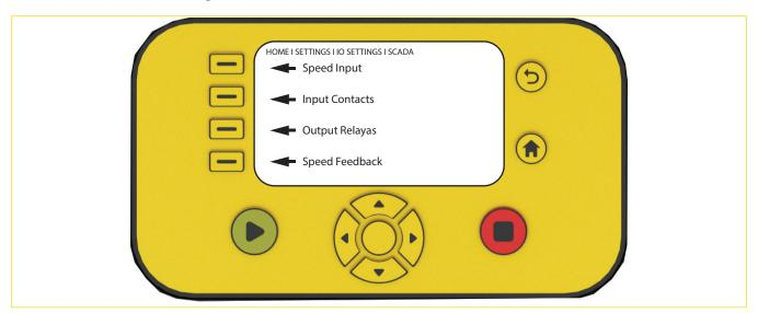
The pump can be configured to accept an analog signal for speed control. The pump can also scale the signal as needed. Speed input displays the scaled value for pump operation according to the the incoming signal value.
