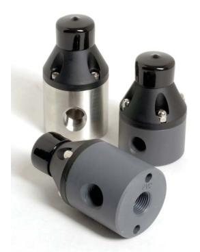
**Griffco M-Series** diaphragm pressure relief valves are designed to protect chemical feed systems from over pressure damage caused by defective equipment or a blockage in the chemical feed line. Robust construction ensures reliability in the rigorous service of municipal and industrial applications. Wetted materials include: **PVC, CPVC, PP, PVDF, PTFE, Halar, 316 SS, A20 and Hastelloy C**. Available sizes: 1/4", 3/8", and 1/2".
